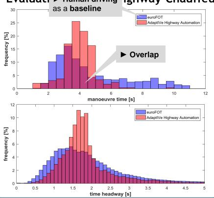
The AdaptIVe Highway-Chauffeur is showing a control capability similar to human driving from euroFOT. Two results stand out:
